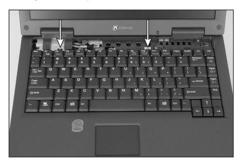
5 Slide the two tabs located on the left end of the bezel under the notebook frame.
