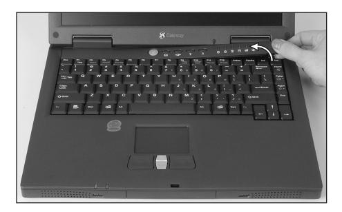
**8** With a small Phillips screwdriver, remove the two keyboard screws and put them in a safe place.
